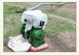
Fig. 24:5HP Disel pump set used to lift water from river tributory for irrigation purpose
